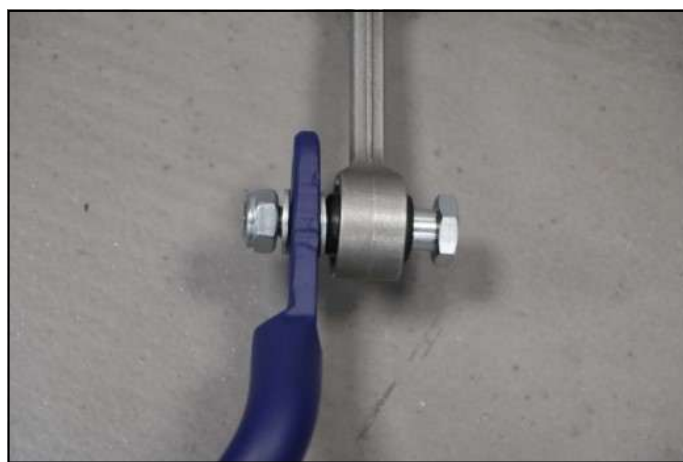
Fig. 2: Tightening of the screw with approx. 50
